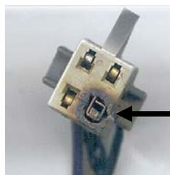
Melted connector caused by heat generated from arcing at connection
