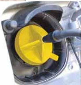
5-year warranty. The Pop-it is perfect for smoke-based leak detection or pressure/vacuum decay EVAP system testing. To use, simply remove the gas cap, pop the Pop-it onto the vehicle's fuel tank neck and connect any smoke machine or leak detection device. *Category: Leak detection.*
